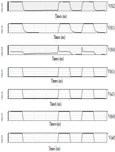
Figure 10: Simulation Waveform of 4 bit Vedic Multiplier Using SERF Adder
