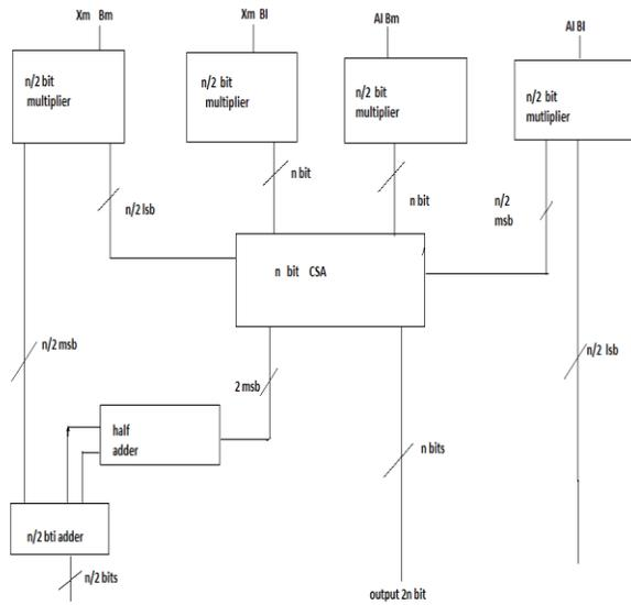
Fig 3:- Complete block diagram for n x n bit Vedic multiplier
