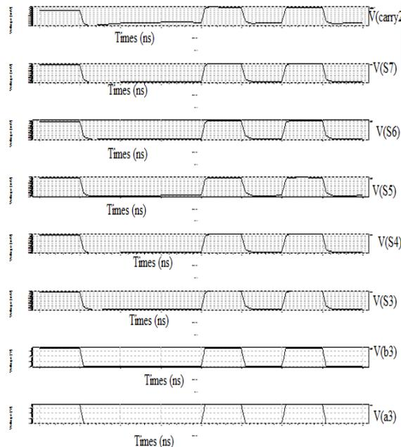
Figure 11: Simulation Waveform of 4 bit Vedic Multiplier Using SERF Adder
