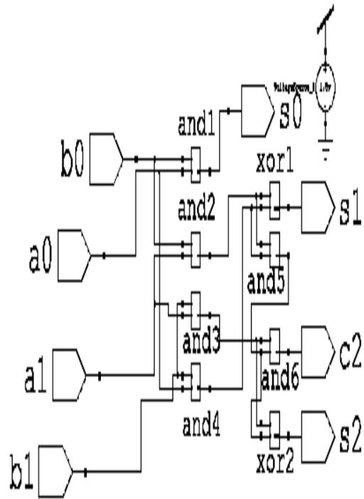
Figure 4: Schematic of 2 bit Vedic Multiplier
