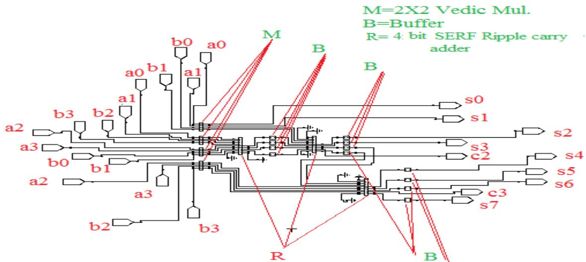
Figure 5: Schematic of 4 – bit Vedic Multiplier using SERF Adder
