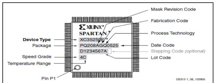
Fig. 2 Spartan 3 QFP package
