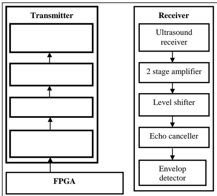
Fig. 1 Block diagram of underwater acoustic modem
