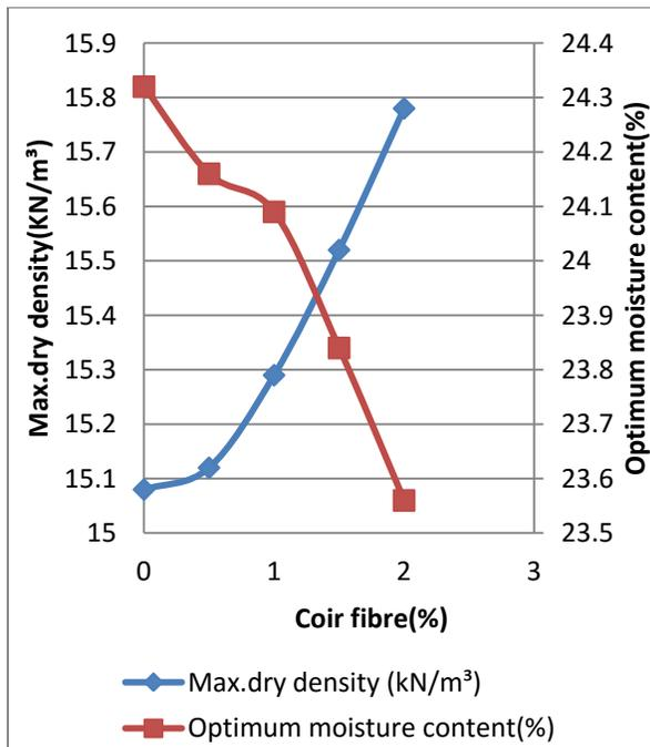
Figure 8: Variation of maximum dry unit weight and optimum moisture content of expansive soil-lime-gypsum mix with varying percentage of coir fibres
