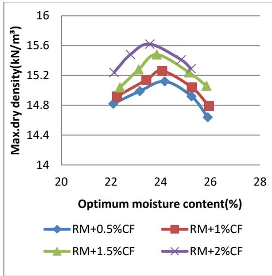
Figure 7: Compaction curves for expansive soil-lime-gypsum mix with varying percentage of coir fibres
