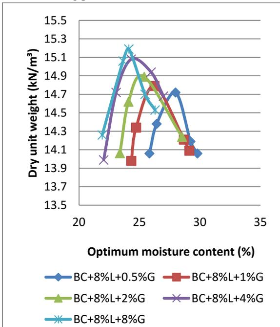
Figure 4: Compaction curves for expansive soil + 8% lime with varying percentage of gypsum
