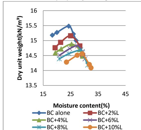
Figure 1: Compaction curves for expansive soil with varying percentage of lime
