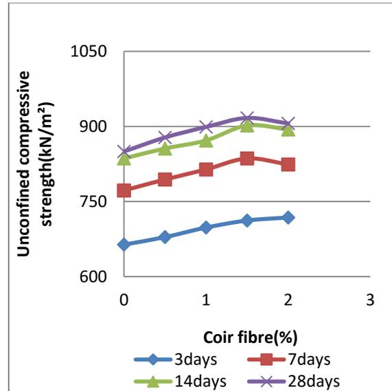
Figure 9: Variation of unconfined compressive strength of expansive soil-lime-gypsum mix with varying percentage of coir fibres and curing period
