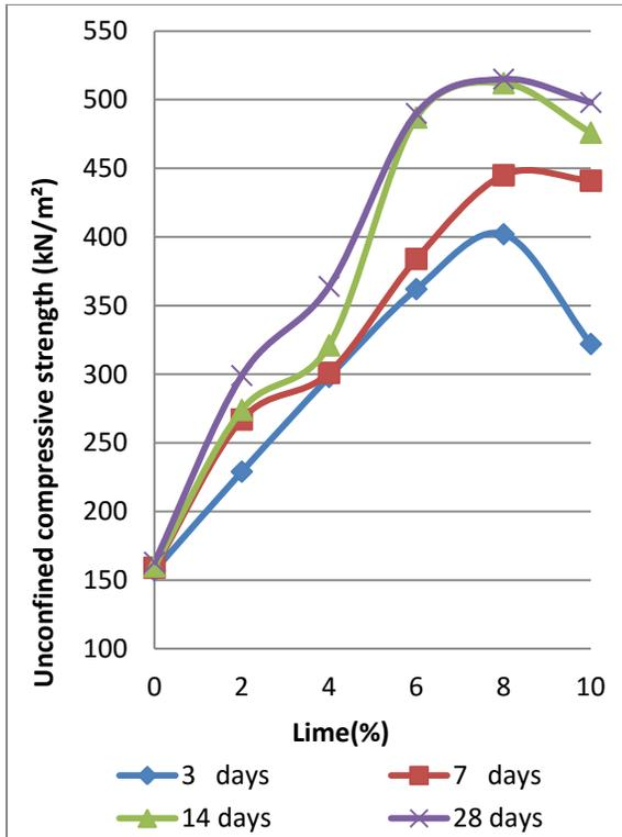
Figure 3: Variation of unconfined compressive strength of expansive soil with varying percentage of lime and curing period
