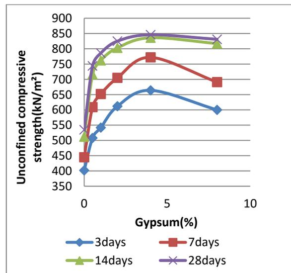
Figure 6: Variation of unconfined compressive strength of expansive soil + 8% lime with varying percentage of gypsum and curing period
