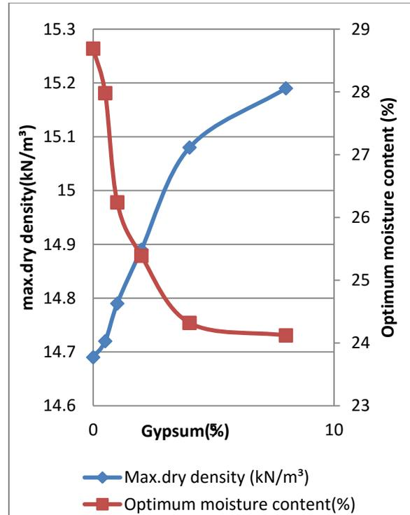
Figure 5: Variation of maximum dry unit weight and optimum moisture content of expansive soil + 8% lime with varying percentage of gypsum
