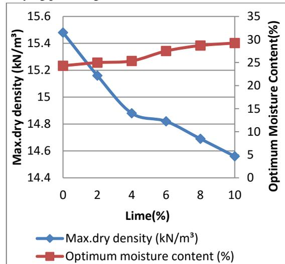
Figure 2: Variation of maximum dry unit weight and optimum moisture content of expansive soil with varying percentage of lime
