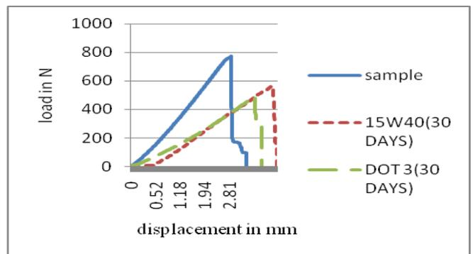
Fig.7: The Effects of Solutions for Bending Specimen (30days)
