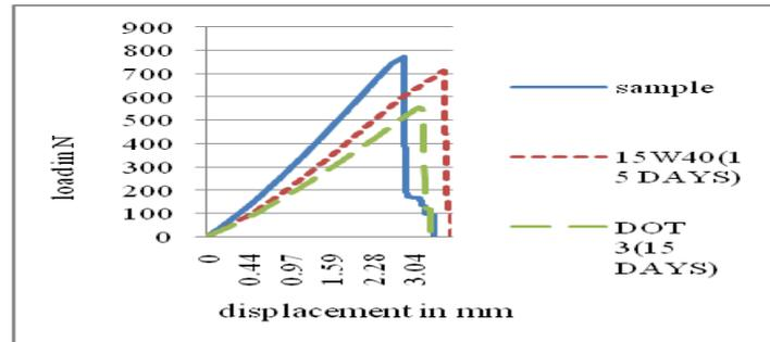
Fig.6: The Effects of Solutions for Bending Specimen (15days)
