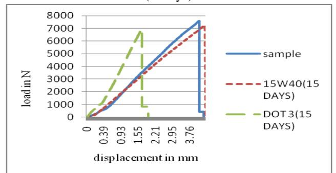
Fig.8: The Effects of Solutions for Tensile Specimen (15days)
