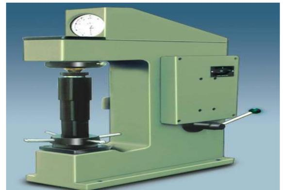
Fig.5: Rockwell Hardness Testing Machine (AL RAS)
