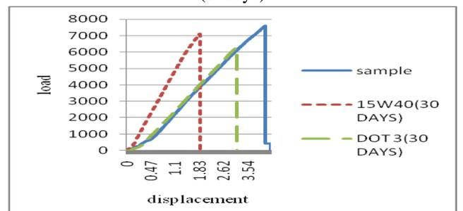
Fig.6.34: The Effects of Solutions for Tensile Specimen (30days)
