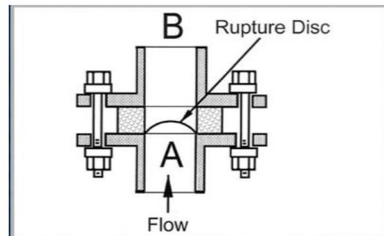
Fig 2: Rupture disk working principle [11]
