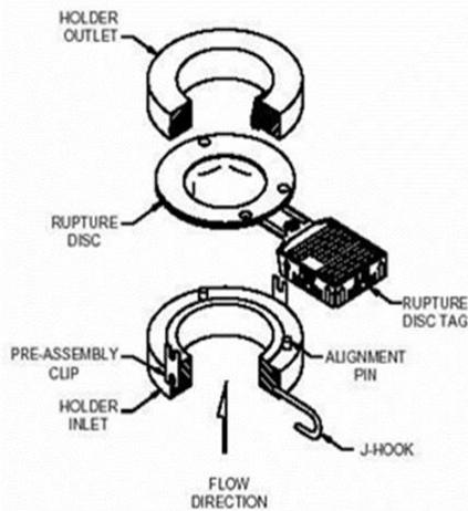
Fig 3: Rupture disc and parts schematic drawing
