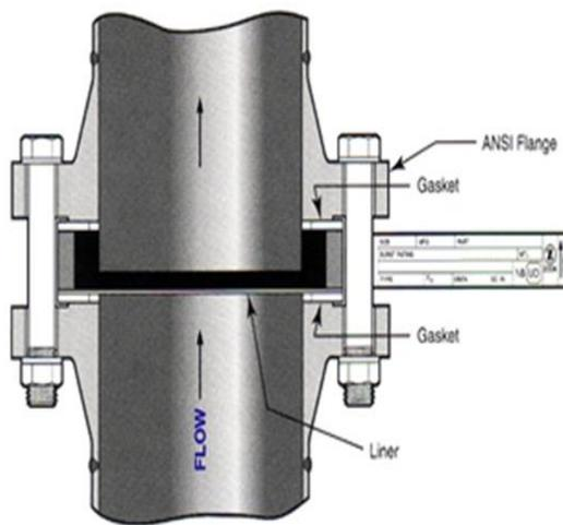
Fig4: Installed rupture disc[13]
