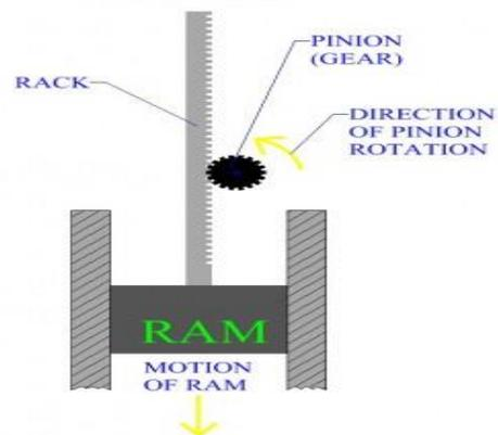
**Fig 7: Rack And Pinion Press**
