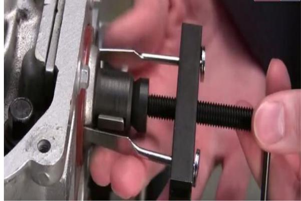
Fig 3: Oil Seal Installation at Workshop
