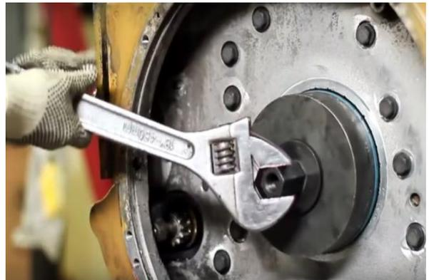
Fig 4: Oil Seal installation of heavy duty Engine
