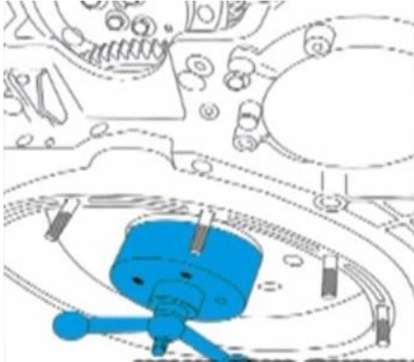
**Fig 5: Oil seal installation tool of Volvo Truck**
