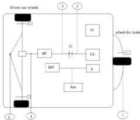
Fig. (2). Topology designing of the proposed vehicle.
