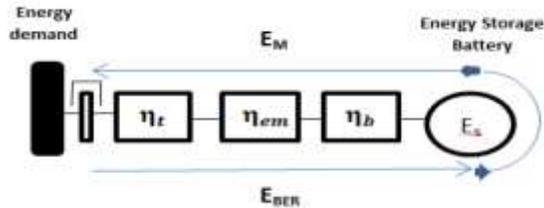
Fig. (1). Schematic diagram of the vehicle power train.
