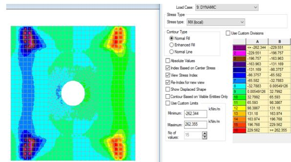
**Fig 10. Maximum bending moment in slab of 20m staging for full condition, Bhuj earthquake**
