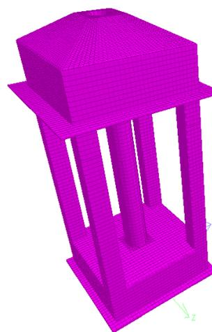
**Fig 2. 3D model of the elevated water tank.**
