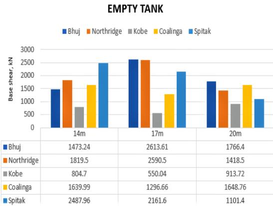
**Fig 7. Base shear comparison for Empty tank**
