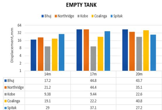
Fig 4. Displacement comparison for Empty tank
