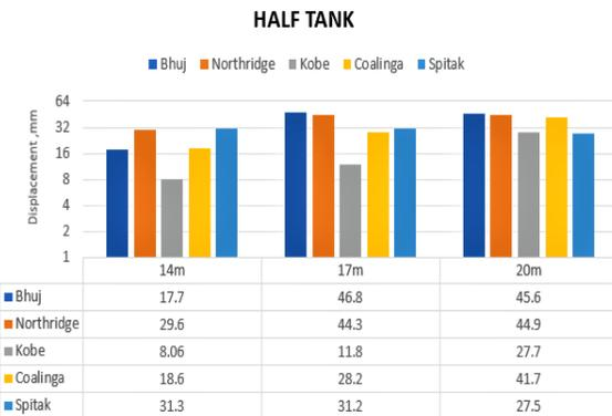
Fig 5. Displacement comparison for Half tank
