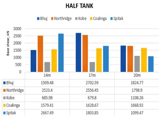
**Fig 8. Base shear comparison for Half tank**
