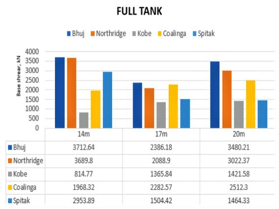
**Fig 9. Base shear comparison for Full tank**
