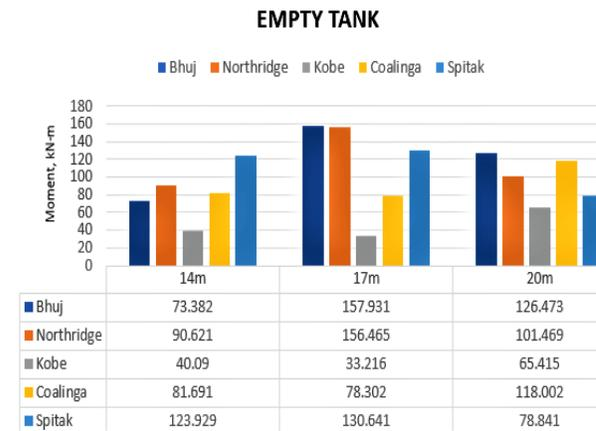
**Fig 11. Bending moment comparison for empty tank**
