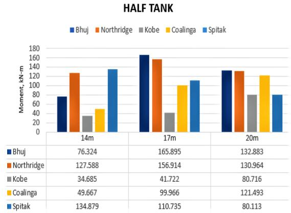
Fig 12. Bending moment comparison for Half tank
