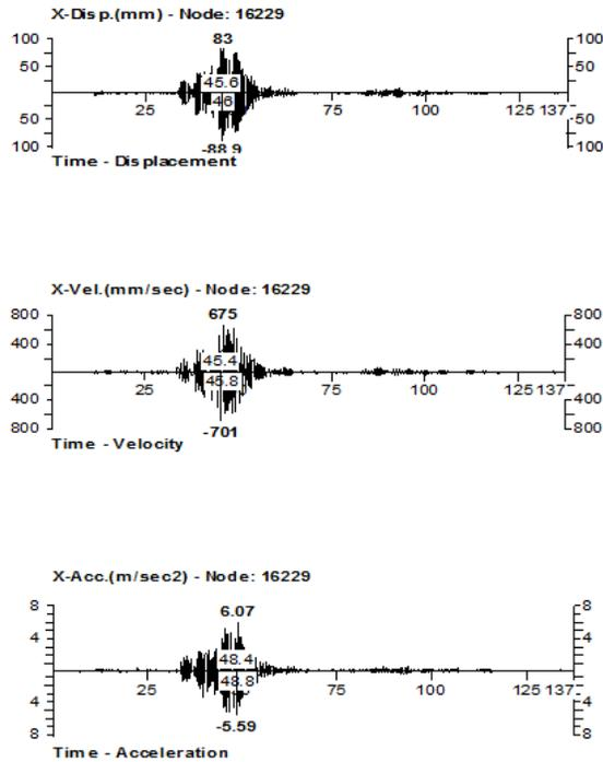
Fig 3. Time History graph of Bhuj earthquake 20m staging under full tank condition
