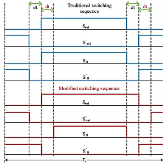
Fig. 7 Delayed dead-time intervals in both converters when current direction is positive
