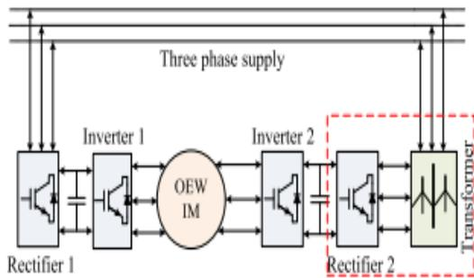
Fig. 1 Conventional open-end winding IM drive topology
