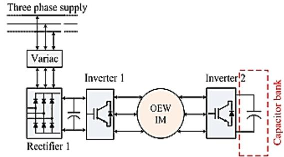
Fig.2 Block diagram of the proposed floating bridge topology.
