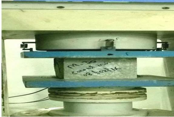
Fig 3: Compressive strength test
