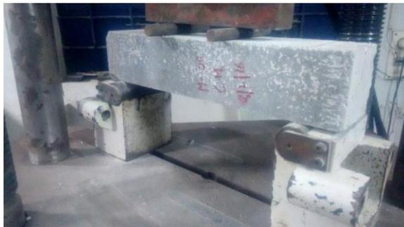
Fig 4: Flexural strength test
