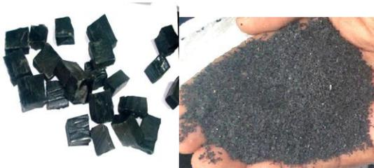
Fig 1: Crumb rubber fragments and powder
