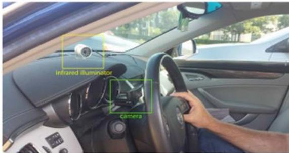
*Fig1: Camera arranged at the steering*
