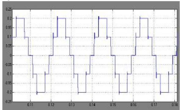
Fig 2. Experimental waveforms for stator current of a 5-level inverter output
