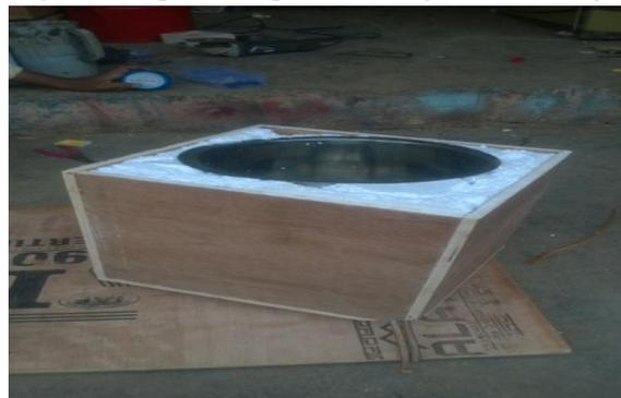
Figure 2: PCM container around the evaporator.
