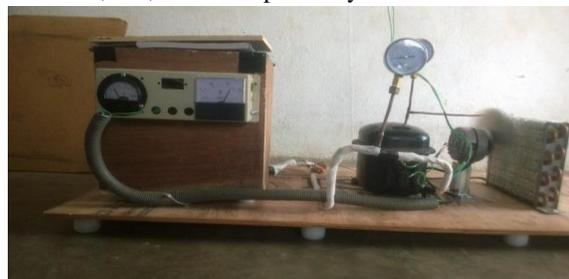
Figure 1: Vapour compression refrigeration test rig
