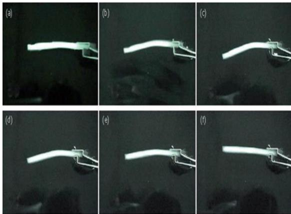
Triple-SME. Upon immersing into hot water, the SMH beam bends downward and then upward.
