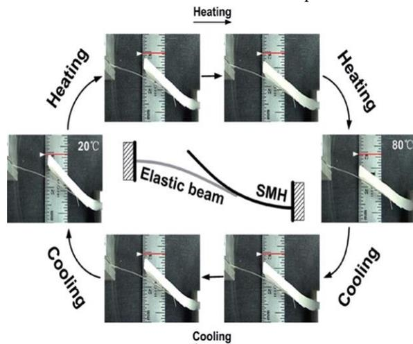
Two-way SME. Upon heating (top half, from left to right), the SMH beam pushes down the elastic beam (see inset for the illustration of set-up). Subsequently, upon cooling (bottom half, from right to left), the elastic beam pushes the SMH beam upward.
