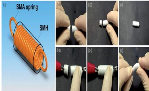
Self-healing of SMH. (a) SMH with an embedded SMA spring inside (illustration); (b1-b2) pulling SMH till fracture; (b3-b4) joule heating SMA coil for self-healing; (c) healed sample; (d) healed sample in bending.
