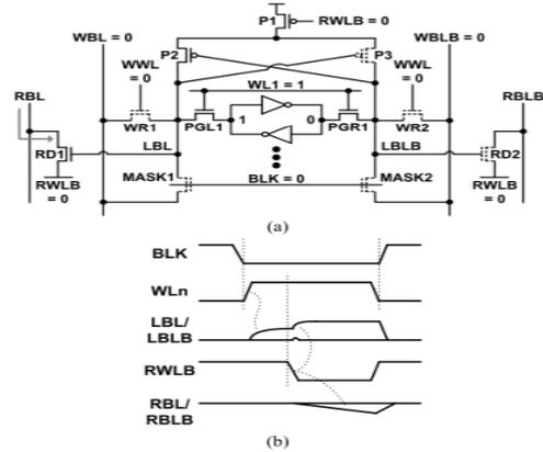
Fig. 4. (a) Read operation and (b) read operational waveform of proposed RAM architecture.
