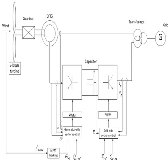
Figure 4. Control diagram of RSC and GSC of grid-connected wind turbine with DFIG
