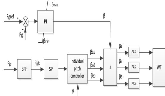
Figure 5. A novel individual pitch control scheme
