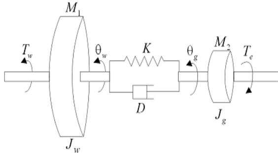
Figure 3. Two-mass model of the drivetrain
