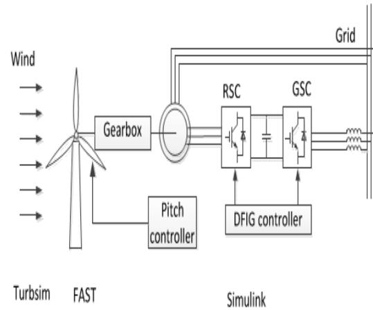
Fig. 2. The overall scheme of the DFIG based wind turbine system
