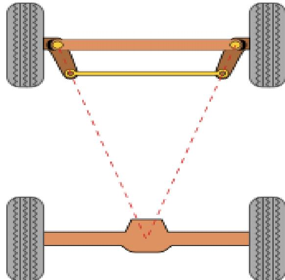
When the vehicle turns, the outer tyre has to turn less than the inner tyre to avoid drag and give good feeling to the driver while cornering at high speed. While turning, the geometry looks like the figure mentioned below.
