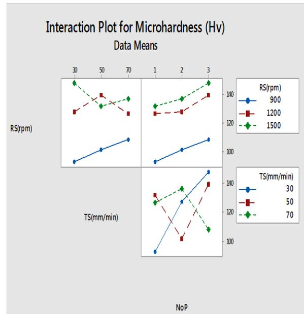
Fig. 5 Interaction Plot for Microhardness (Data Means)
