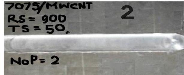
Fig. 2 AA7075/MWCNT SMMC billet from FSP Exp - 2
