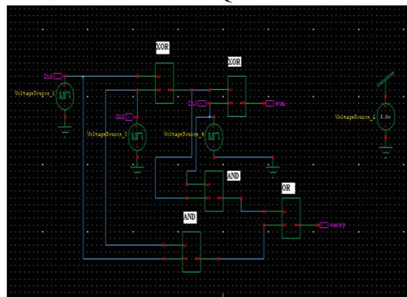
TRANSISTOR LEVEL CIRCUIT FOR FULL ADDER IN GDI TECHNIQUE
