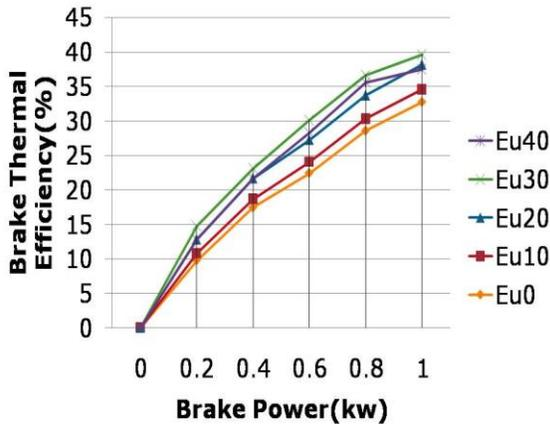
Fig.3 B.Th.η Vs Brake Power
