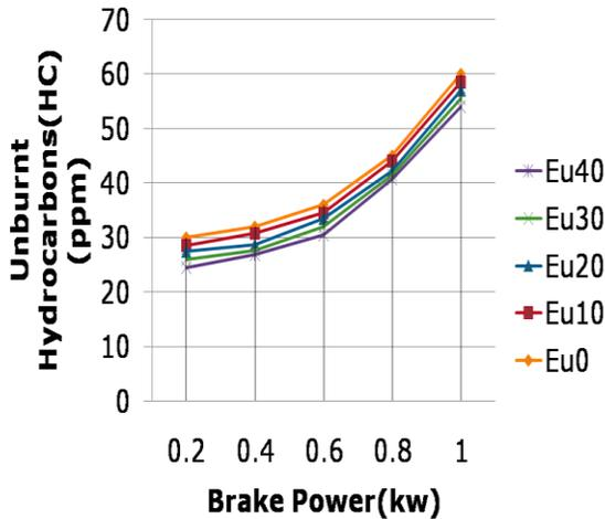
Fig. 8 Unburnt Hydrocarbons Vs Brake Power
