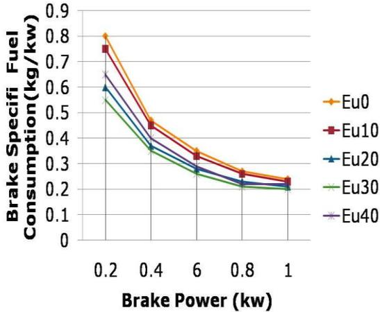
Fig.4 Bsfc Vs Brake Power
