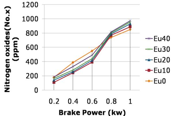
Fig. 7 Nitrogen Oxides Vs Brake Power
