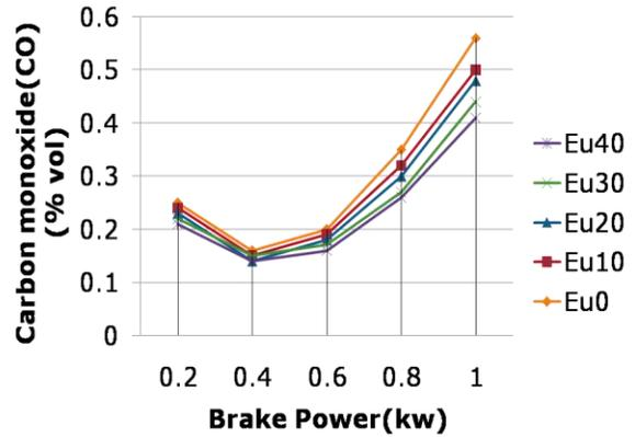
Fig. 5 Carbon Monoxide Vs Brake Power
