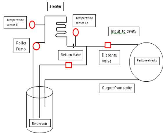
Figure 1 schematic diagram of custom made HIPEC system
