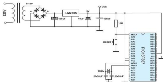
All the electronic component starting from diode to Intel IC's only work with a DC supply rating from  $\pm 5V$  to  $\pm 12V$ . We are utilizing for the same, the cheapest and commonly available energy sources of 230V-50Hz supply and stepping down, rectifying, filtering and regulating the voltage, depending upon over requirements. Fig 4.1 shows the circuit diagram for power supply say 5V and 12V as per requirements.
