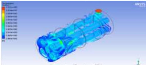
Figure 4.31 Cold Fluid Outlet Temperature for 5 Baffles Shell and Tube Heat Exchanger at 15°C Cold Fluid Inlet Temperature
