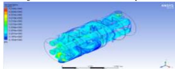
Figure 4.26 Hot Fluid Outlet Temperature for 5 Baffles Shell and Tube Heat Exchanger at 10°C Cold Fluid Inlet Temperature
