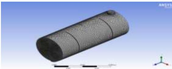
Figure 3.5 Mesh generated of 3 baffles shell and tube heat exchanger
