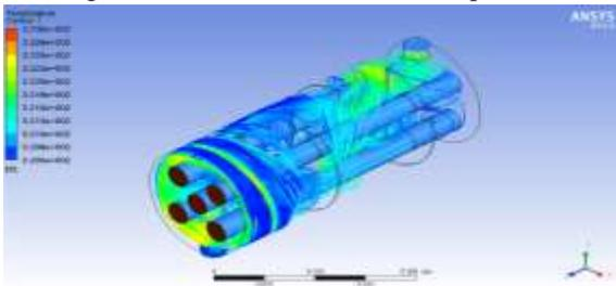
Figure 4.22 Hot Fluid Outlet Temperature for 4 Baffles Shell and Tube Heat Exchanger at 20°C Cold Fluid Inlet Temperature
