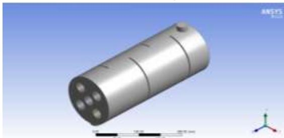
Figure 3.2 Geometry of 4 Baffles Shell and Tube Heat Exchanger
