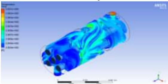
Figure 4.3 Cold Fluid Outlet Temperature for 3 Baffles Shell and Tube Heat Exchanger at 10°C Cold Fluid Inlet Temperature
