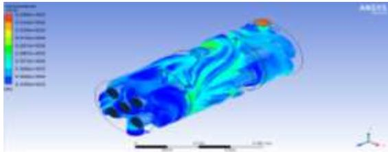
Figure 4.11 Cold Fluid Outlet Temperature for 3 Baffles Shell and Tube Heat Exchanger at 20°C Cold Fluid Inlet Temperature
