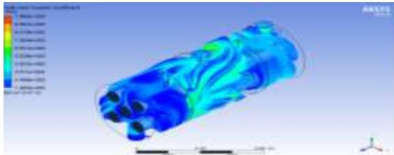
Figure 4.13 Wall Heat Transfer Coefficient for 3 Baffles Shell and Tube Heat Exchanger at 20°C Cold Fluid Inlet Temperature
