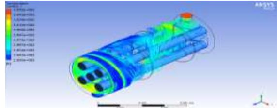
Figure 4.23 Cold Fluid Outlet Temperature for 4 Baffles Shell and Tube Heat Exchanger at 20°C Cold Fluid Inlet Temperature
