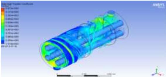
Figure 4.21 Wall Heat Transfer Coefficient for 4 Baffles Shell and Tube Heat Exchanger at 15°C Cold Fluid Inlet Temperature
