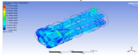
Figure 4.36 Turbulence Eddy Dissipation for 5 Baffles Shell and Tube Heat Exchanger at 20°C Cold Fluid Inlet Temperature
