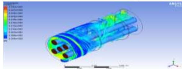
Figure 4.18 Hot Fluid Outlet Temperature for 4 Baffles Shell and Tube Heat Exchanger at 15°C Cold Fluid Inlet Temperature
