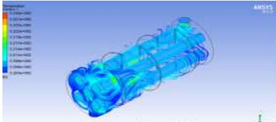
Figure 4.30 Hot Fluid Outlet Temperature for 5 Baffles Shell and Tube Heat Exchanger at 15°C Cold Fluid Inlet Temperature
