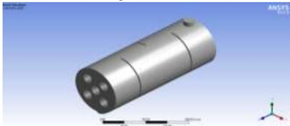
Figure 3.1 Geometry of 3 Baffles Shell and Tube Heat Exchanger
