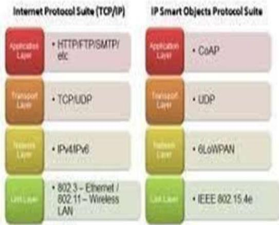
Fig 3. TCP/IP STACK and IP Smart Objects Protocols Stack
