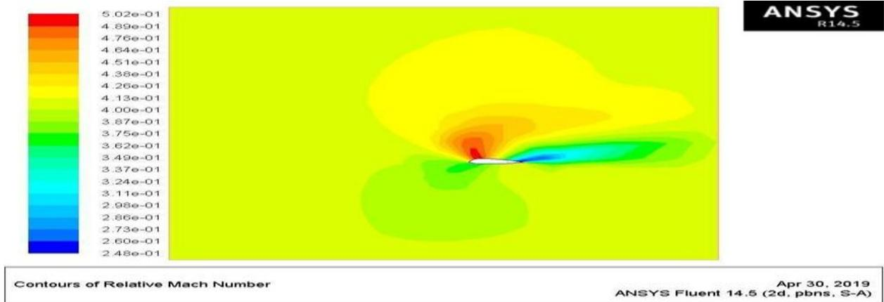
Figure 7: Relative Mach number contour at AOA is 10 degree.
