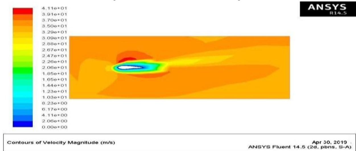
Figure 5: Velocity contour at AOA is 10 degree.
