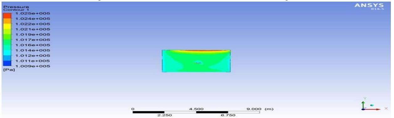
Figure 8: Pressure contour at front rotor.
