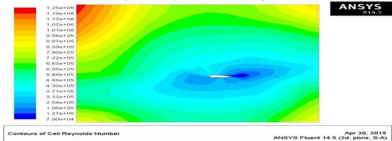
Figure 6 Reynold's number contour at AOA is 10 degree
