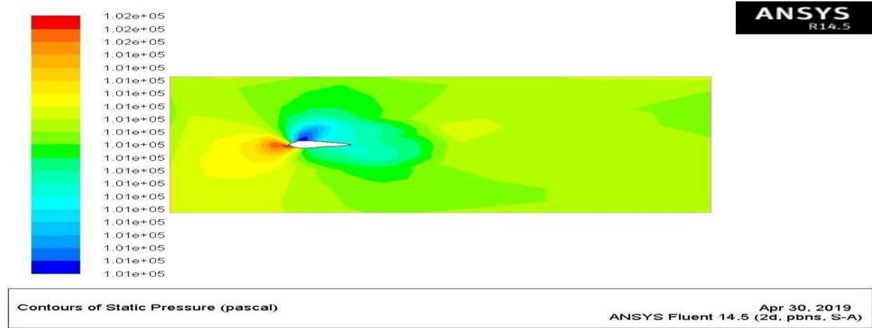
Figure 4: Pressure contour at AOA is 10 degree.
