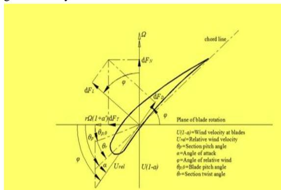
Figure 1: Schematic diagram of blade, angle of attack, pitch angle etc. [8]
