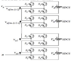
Fig.1.Single-phase structure of a cascaded H-bridge inverter
