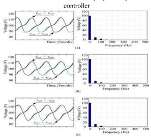
Fig.12.Capacitor voltages of all SMs in one phase leg (simulation results). With PI controller only. (b) With MAF + PI controller. (c) With MAF + PI controller +proposed repetitive controller. reduced, indicating better command-following and disturbance rejection at these frequencies.
