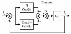
Fig.7..Control structure of pi based controller In [15], a repetitive controller is paralleled with the PI controller to improve harmonic suppression. The resulted control structure is shown in Fig. 5. Such a parallel configuration of a repetitive controller and
