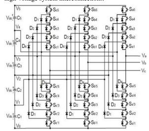
Fig.3.Three-phase six-level structure of a diodeclamped inverter
