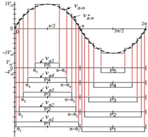
Fig.2.Output phase voltage waveform of an 11-level cascade inverter with 5 separate dc sources
