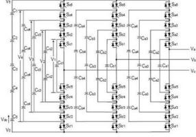
Fig.4.Three-phase six-level structure of a flying capacitor inverter
