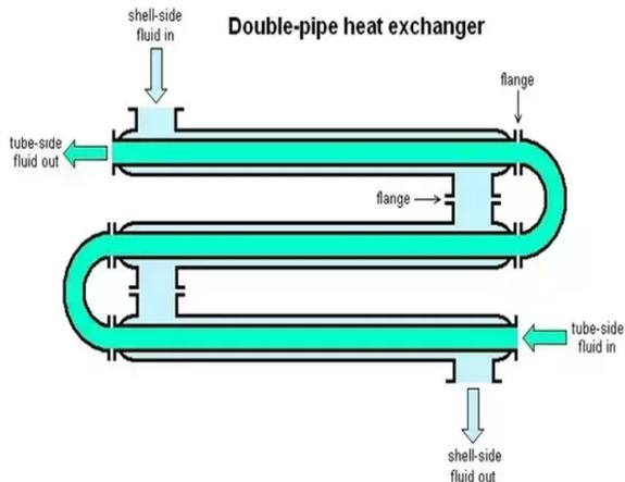
Fig. 4: U-type double pipe heat exchanger
