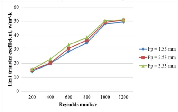
Fig. 18: Effect of varying fin pitch on heat transfer coefficient variation for Wavy fin In-line Configuration
