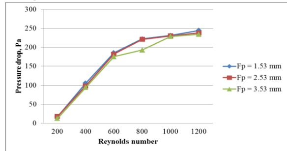
Fig. 36: Effect of varying fin tube pitch on pressure drop variation for wavy fin staggered configuration
