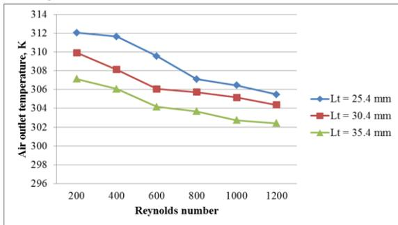
Fig. 10: Effect of varying transverse tube pitch on air outlet temperature variation for Wavy fin In-line Configuration
