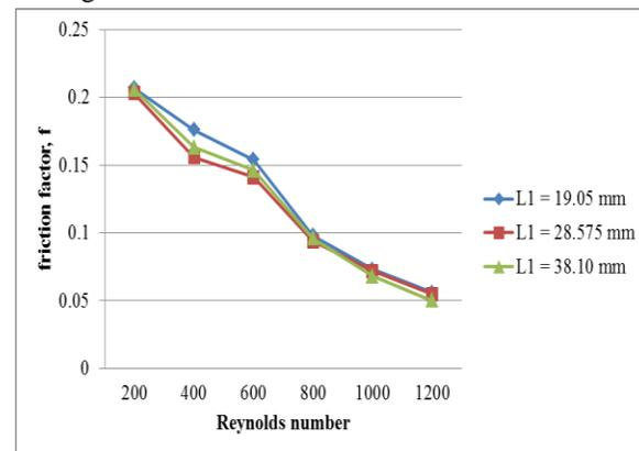
Fig. 8: Effect of varying longitudinal tube pitch on friction factor variation for Wavy fin In-line Configuration
