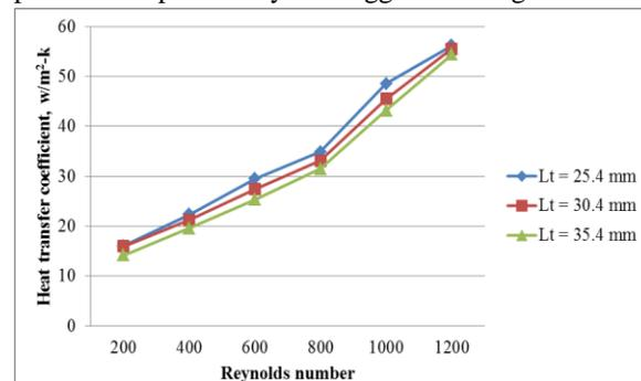
Fig. 31: Effect of varying longitudinal tube pitch on heat transfer coefficient for wavy fin staggered configuration
