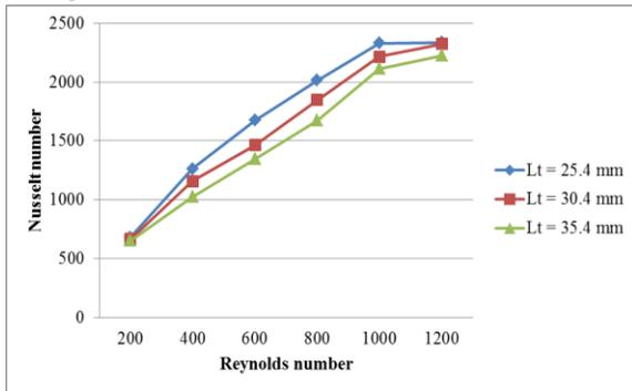
Fig. 32: Effect of varying longitudinal tube pitch on Nusselt number for wavy fin staggered configuration
