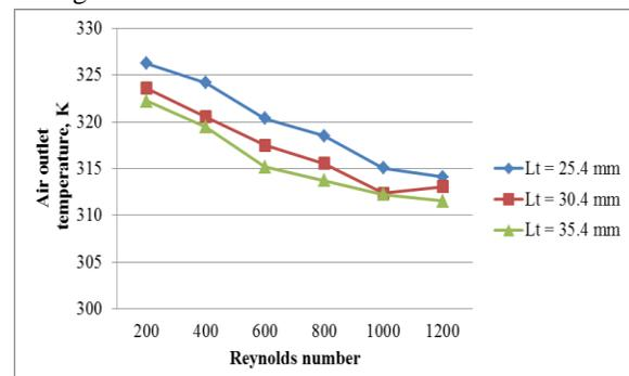
Fig. 29: Effect of varying longitudinal tube pitch on air outlet temperature for wavy fin staggered configuration
