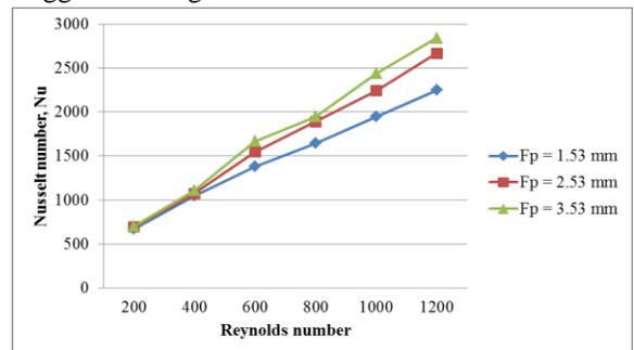
Fig. 38: Effect of varying fin tube pitch on Nusselt number variation for wavy fin staggered configuration
