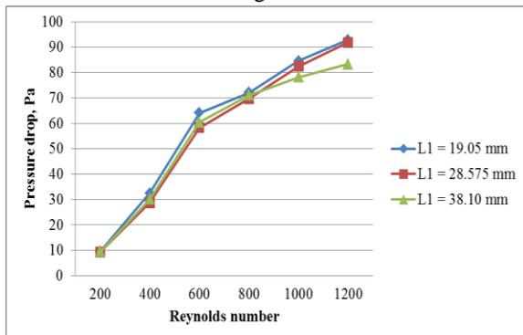
Fig. 5: Effect of varying longitudinal tube pitch on pressure drop variation for Wavy fin In-line Configuration
