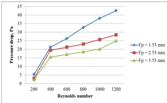
Fig. 17: Effect of varying fin pitch on pressure drop variation for Wavy fin In-line Configuration
