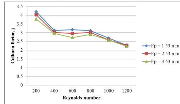
Fig. 21: Effect of varying fin pitch on Colburn factor variation for Wavy fin In-line Configuration
