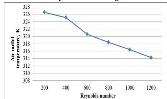
Fig. 22: Air outlet temperature variation for wavy fin staggered configuration
