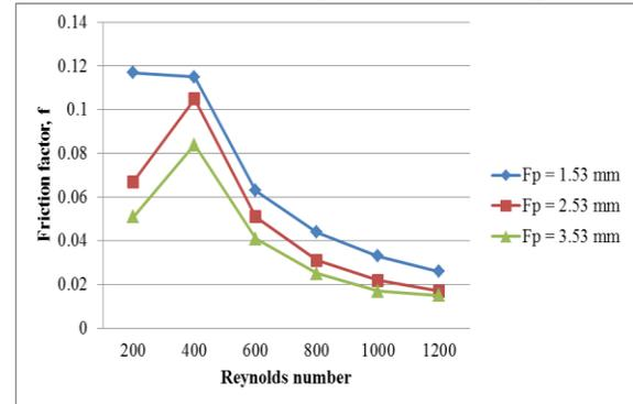
Fig. 20: Effect of varying fin pitch on friction factor variation for Wavy fin In-line Configuration
