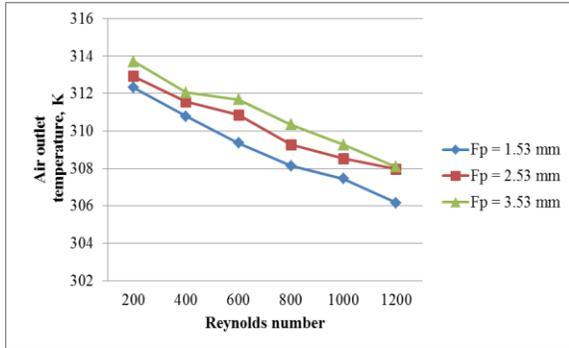
Fig. 16: Effect of varying fin pitch on air outlet temperature variation for Wavy fin In-line Configuration
