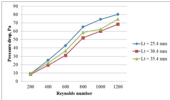
Fig. 11: Effect of varying transverse tube pitch on pressure drop variation for Wavy fin In-line Configuration
