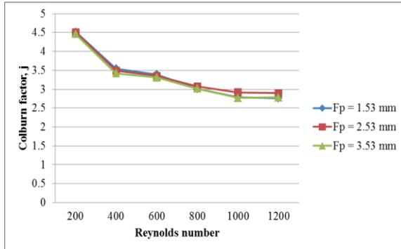
Fig. 40: Effect of varying longitudinal tube pitch on colburn factor variation for wavy fin staggered configuration
