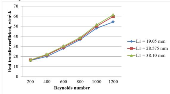
Fig. 25: Effect of varying longitudinal tube pitch on heat transfer coefficient variation for wavy fin staggered configuration
