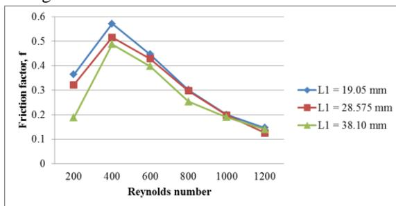
Fig. 27: Effect of varying longitudinal tube pitch on friction factor variation for wavy fin staggered configuration
