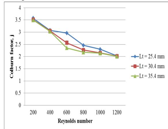
Fig. 15: Effect of varying transverse tube pitch on Colburn factor variation for Wavy fin In-line Configuration
