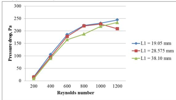
Fig. 24: Effect of varying longitudinal tube pitch on pressure drop variation for wavy fin staggered configuration
