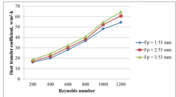
Fig. 37: Effect of varying longitudinal tube pitch on heat transfer coefficient variation for wavy fin staggered configuration
