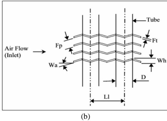
Fig. 3: Nomenclature used with respect to inline wavy-fin and wavy-fin staggered configuration
