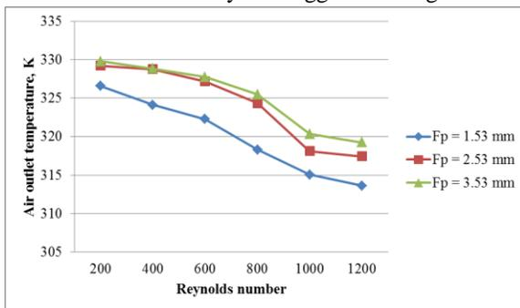
Fig. 35: Effect of varying fin tube pitch on air outlet temperature variation for wavy fin staggered configuration
