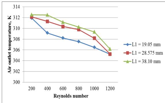
Fig. 4: Effect of varying longitudinal tube pitch on air outlet temperature variation for Wavy fin In-line Configuration
