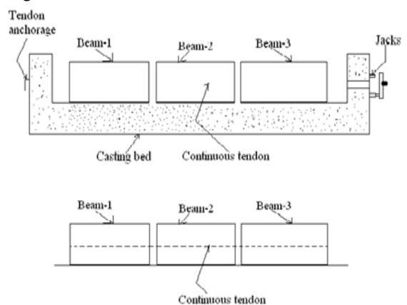
Fig. Hoyer's Long Line System of Pre-tensioning
