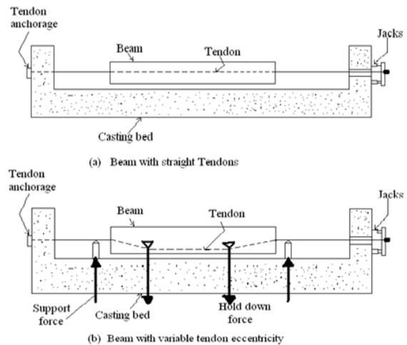
Fig .Method of Pre-tensioning
