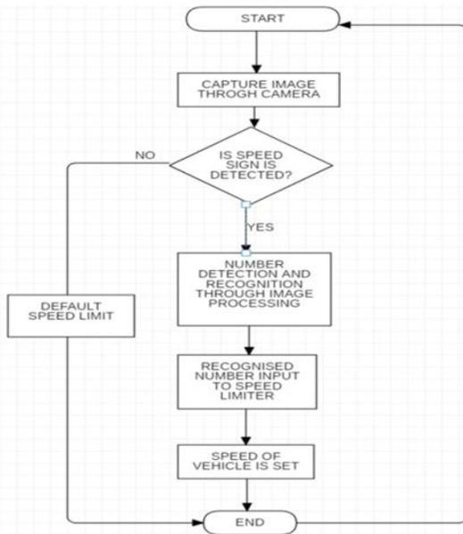
Fig. 2. Flowchart of Speed Control
