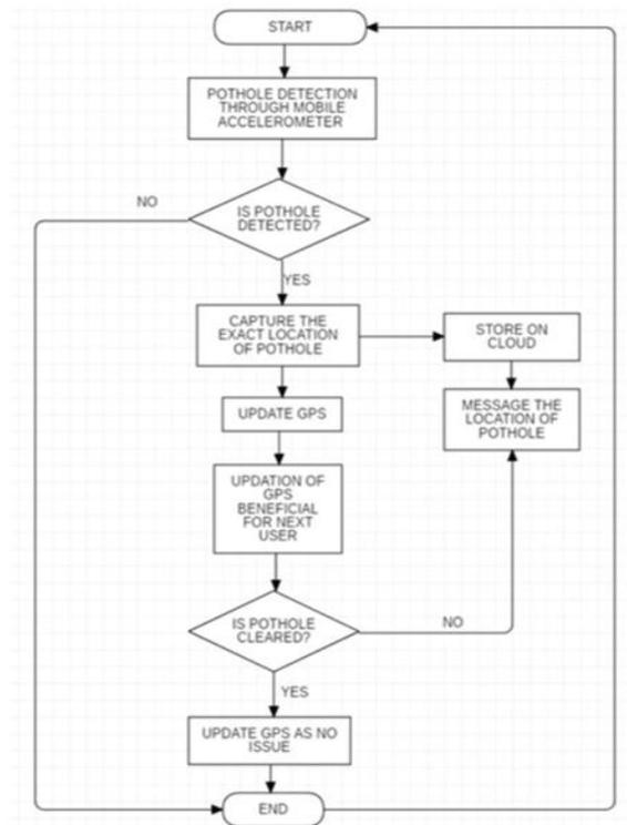
Fig. 3. Flowchart of Pothole Detection System
