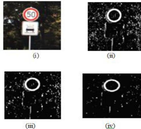
Fig. 5 The speed-limit sign maintains its shape under different thresholds. (i) Original image. (ii.) The preprocessed image. (iii.) Threshold = 150. (iv.) Threshold = 250.
