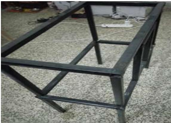
Construction machine consists of stand, bearing support plates, nuts and bolts. Frame is the supporting member which provides support for components like bearing, shaft, blades, belt, pulley etc. In order to get the required strength, two plates (Bearing support blades) are fixed with the help of nut and bolts. The machine frame with a size of 275
