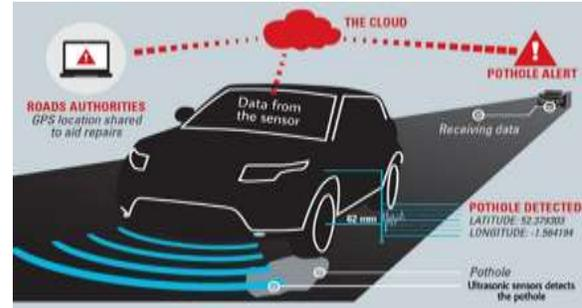
Fig.5: Pothole detection system
