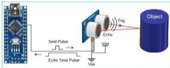
Fig.3: Working of Ultrasonic sensor
