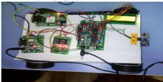
Fig.8: Working model of the pothole system
