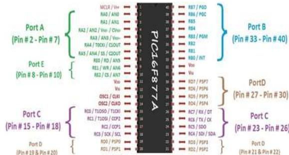
Fig.2: Pin diagram of PIC 16F877A
