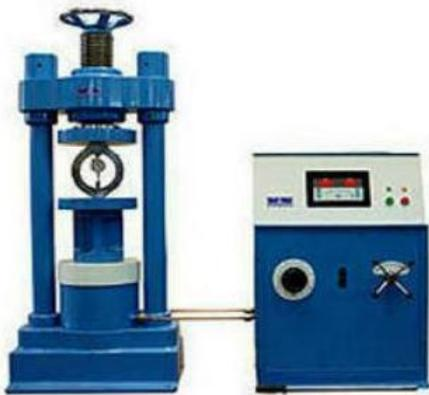
A 2000 kN digital compressive testing machine issued for determine the compressive strength of hardened concrete as per the requirement of IS 516-1959 using standard 150mm\*150mm cubes.
