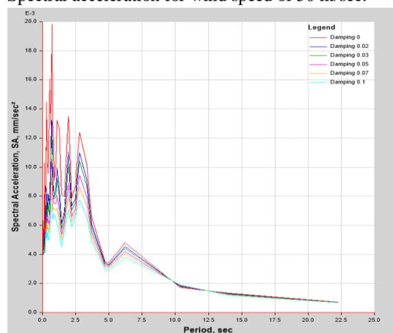
Spectral acceleration for wind speed of 90 m/sec.
