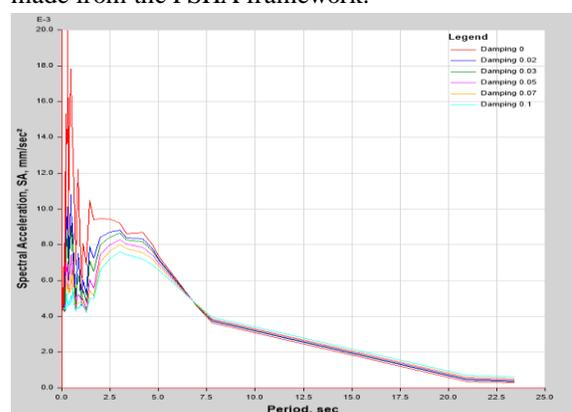
Spectral acceleration for wind speed of 50 m/sec.
