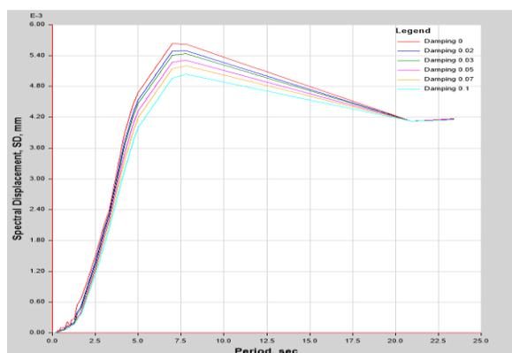
Spectral displacement with wind speed of 90 m/sec.
