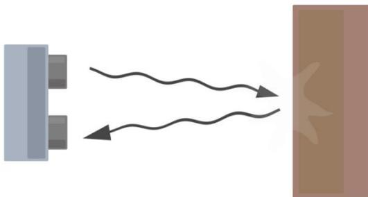
Figure 4 Diagram of the basic ultrasonic sensor operation
