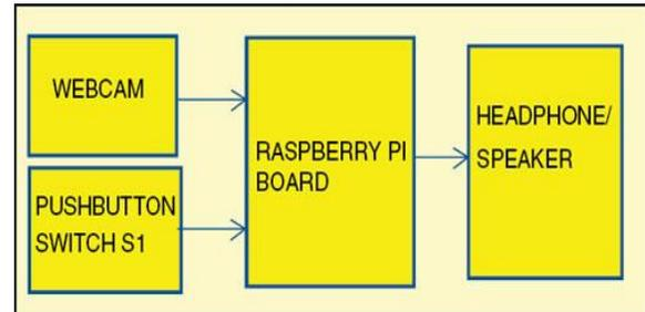
Figure. 5.: Block diagram of the See and Speak system
