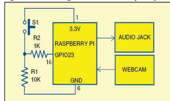
Figure. 6: Circuit connection to Raspi board
