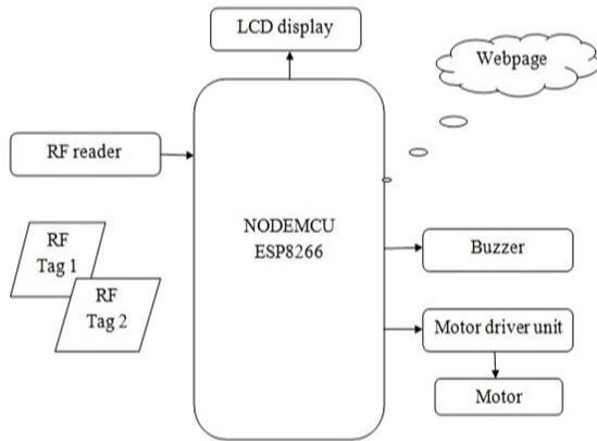
Figure 1 Block Diagram of Proposed Toll Gate System
