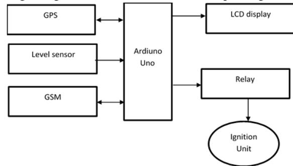
Figure 2 block diagram of GSM based vehicle theft detection and automatic ignition cutoff system
