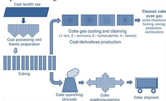
Fig. 1: The basic scheme of coking plant
