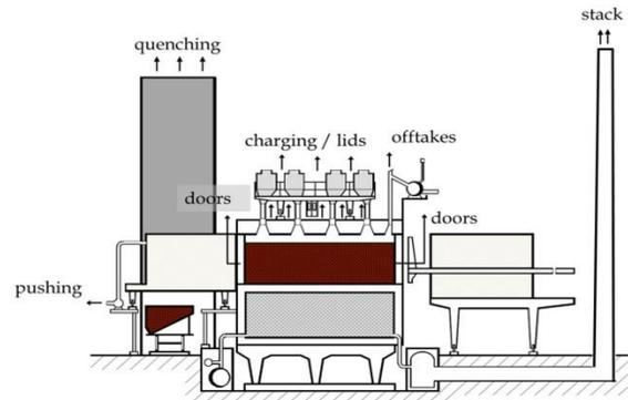
Fig. 2: Schematic drawing of typical emission sources at a conventional coking plant
