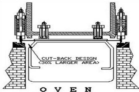
Fig. 7: Coke Oven door cross section view new design diaphragm
