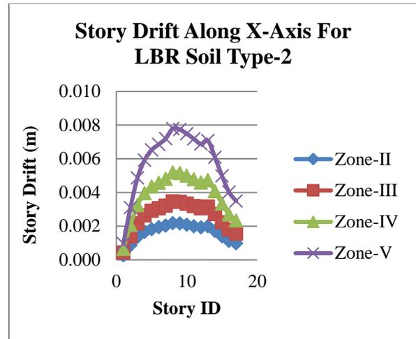
Graph 17: Story Drift along X-Axis with LBR with Soil Type-2.
