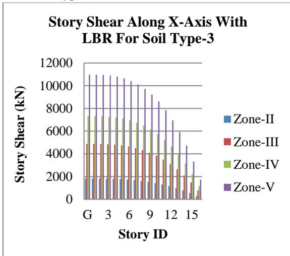
Graph 12: Story Shear along X-Axis for LBR for Soil Type-3.
