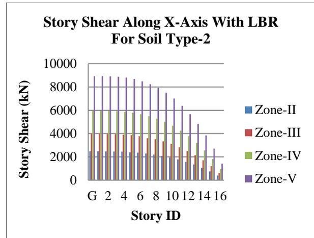
Graph 5: Story Shear along X-Axis for LBR for Soil Type-2.
