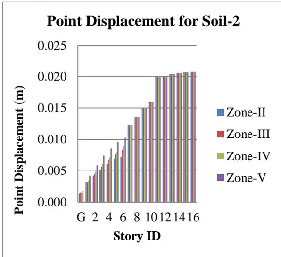
Graph 29: Point Displacement for LBR Support with Soil Type-2.
