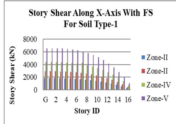
Graph 1: Story Shear along X-Axis for Fixed Support for Soil Type-1.
