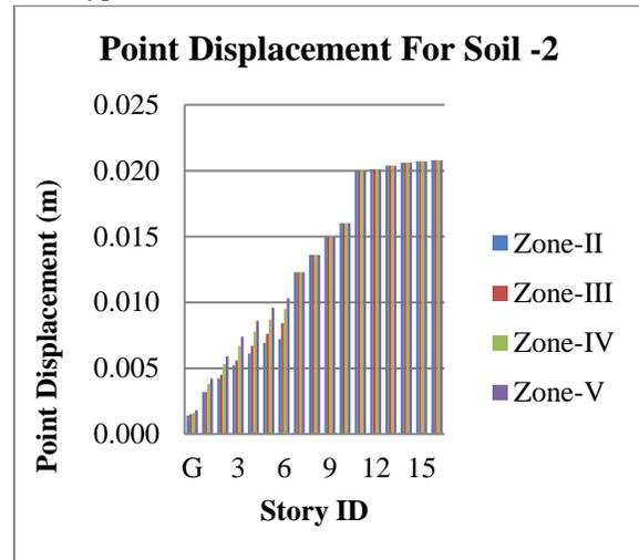
Graph 25: Story Displacement for Fixed Support with Soil Type-2.
