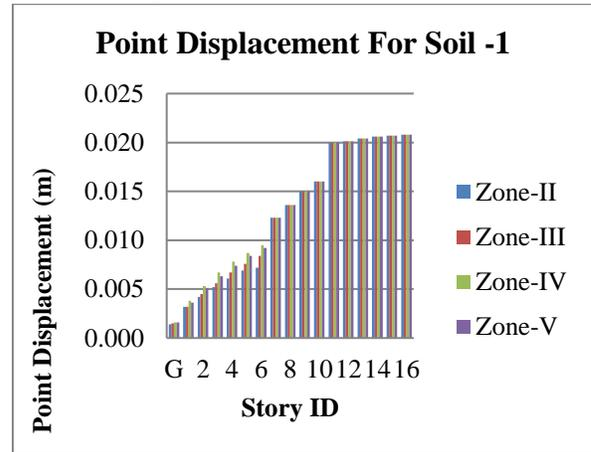
Graph 23: Story Displacement for Fixed Support with Soil Type-1.
