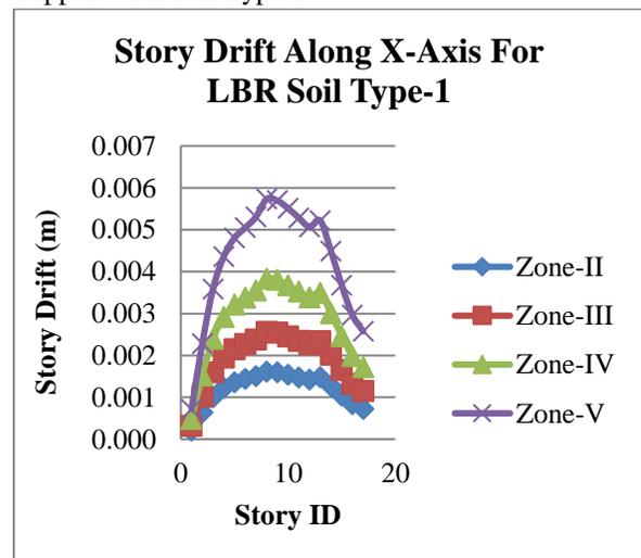
Graph 15: Story Drift along X-Axis with LBR with Soil Type-1
