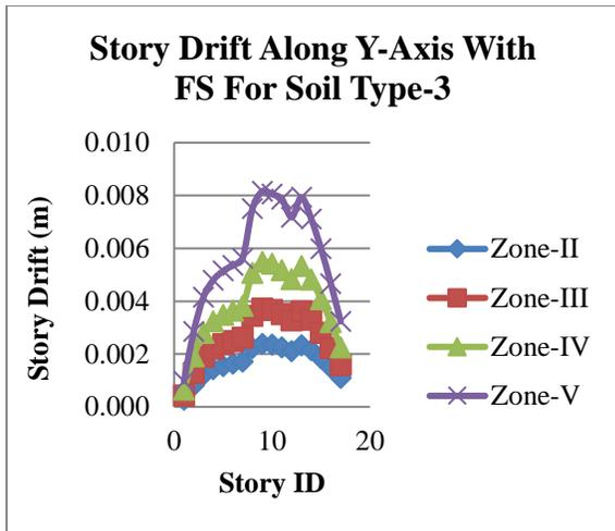
Graph 22: Story Drift along Y-Axis with Fixed Support with Soil Type-3
