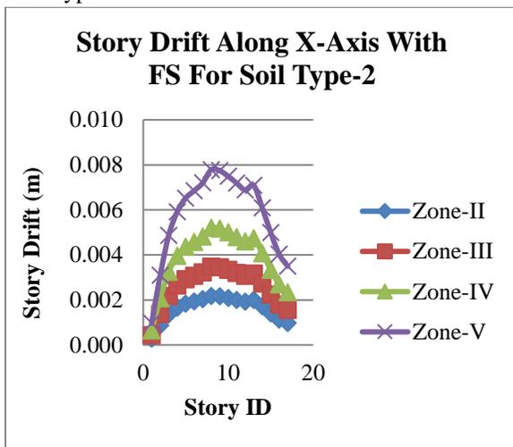
Graph 18: Story Drift along X-Axis with Fixed Support with Soil Type-2
