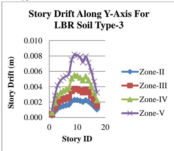
Graph 26: Story Drift along Y-Axis with LBR with Soil Type-3.
