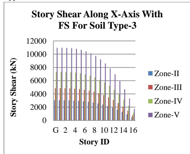
Graph 9: Story Shear along X-Axis for Fixed Support with Soil Type-3.
