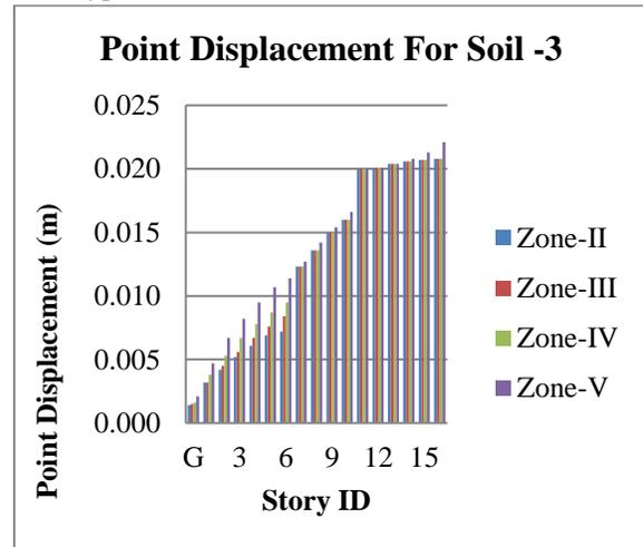
Graph 27: Story Displacement for Fixed Support with Soil Type-3.
