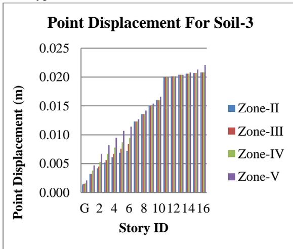
Graph 30: Point Displacement for LBR Support with Soil Type-3.
