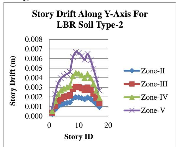
Graph 19: Story Drift along Y-Axis with LBR with Soil Type-2.
