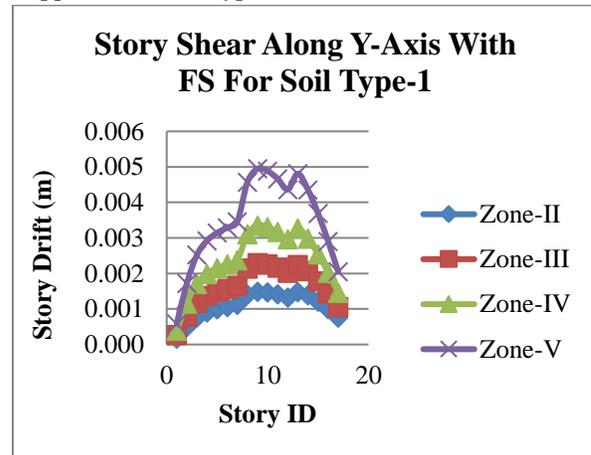
Graph 13: Story Drift along Y-Axis with Fixed Support with Soil Type-1
