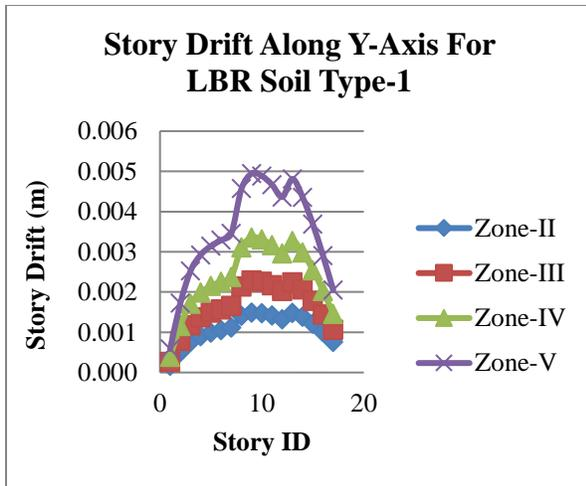
Graph 16: Story Drift along Y-Axis with LBR with Soil Type-1
