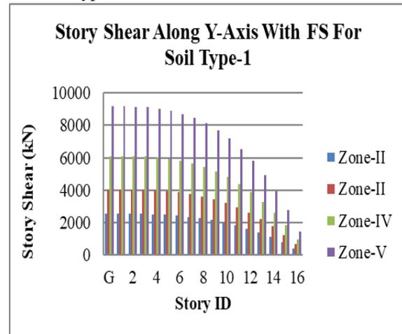
Graph 2: Story Shear along Y-Axis for Fixed Support for Soil Type-1.
