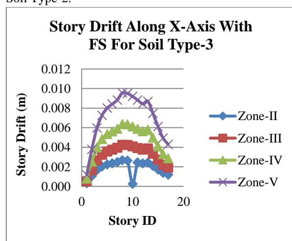
Graph 21: Story Drift along X-Axis with Fixed Support with Soil Type-3
