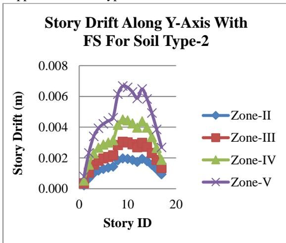
Graph 20: Story Drift along Y-Axis with Fixed Support with Soil Type-2
