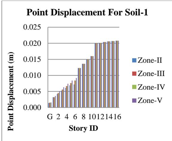
Graph 28: Point Displacement for LBR Support with Soil Type-1.
