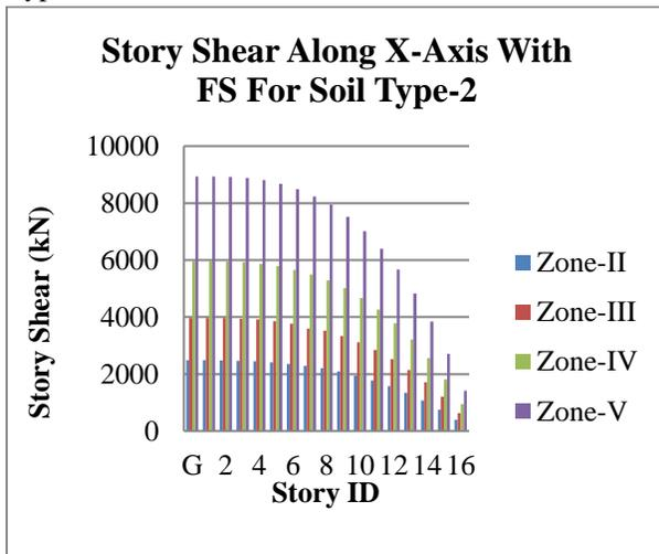
Graph 6: Story Shear along X-Axis for Fixed Support with Soil Type-2.
