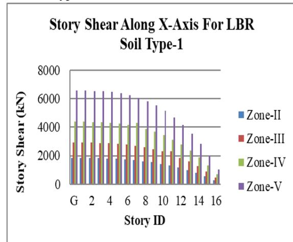
Graph 3: Story Shear along X-Axis for LBR for Soil Type-1.
