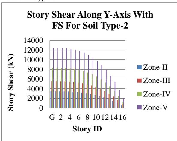
Graph 8: Story Shear along Y-Axis for Fixed Support with Soil Type-2.
