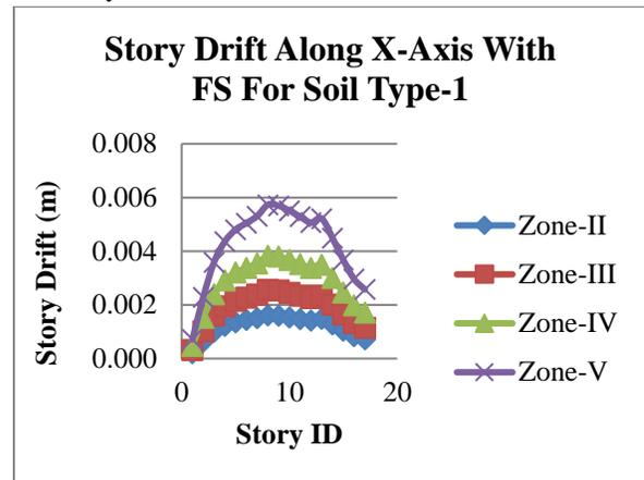
Graph 11: Story Drift along X-Axis with Fixed Support with Soil Type-1
