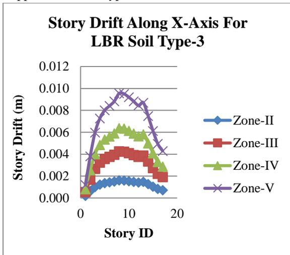
Graph 24: Story Drift along X-Axis with LBR with Soil Type-3.
