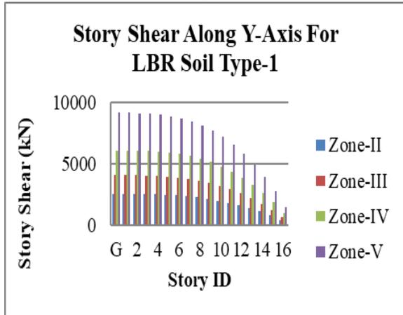
Graph 4: Story Shear along Y-Axis for LBR for Soil Type-1.
