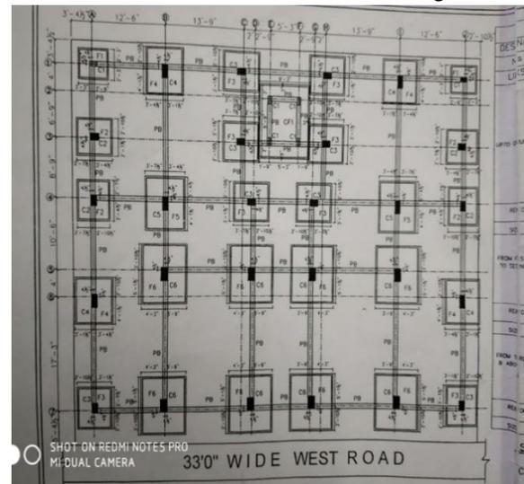
FIG 2: Column framing with center to centre distances between the columns
