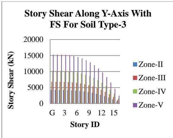
Graph 10: Story Shear along Y-Axis for Fixed Support with Soil Type-3.
