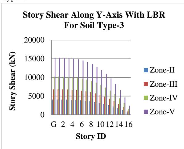
Graph 14: Story Shear along Y-Axis for LBR for Soil Type-3
