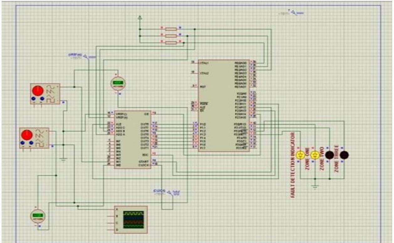
Fig. 6. Indicated and located fault at zone I
