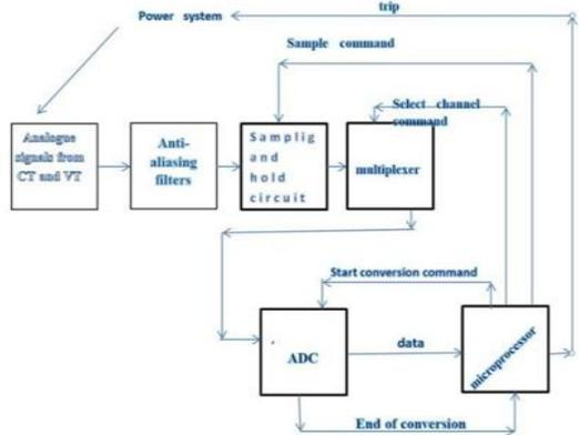
Fig. 1. Block diagram of numerical relay. [4]
