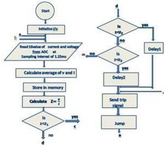
Fig. 2. Flowchart for Main Function
