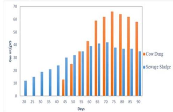
Fig. 5: Comparison of Biogas Production in the Reactor with Sewage Sludge and Cow Dung as Inoculum
