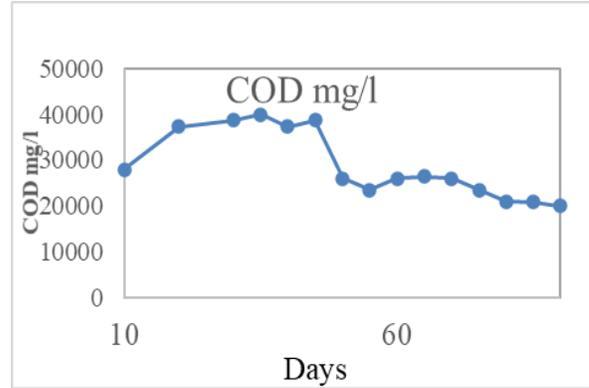
Fig. 4: Variation of COD for Sewage Sludge as Inoculum
