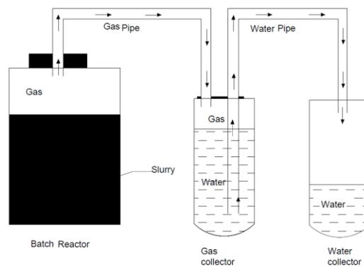
Fig. 1: Schematic Representation of Experimental Setup
