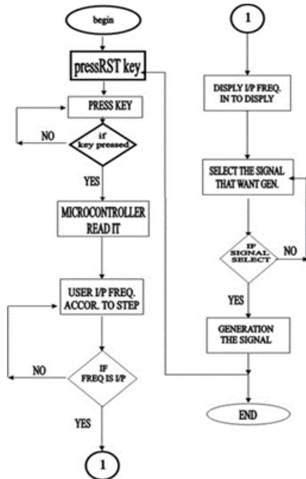
Figure 7 : Signal generator implemented by using one microcontroller
