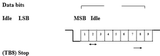
Figure 4: Asynchronous 9-bit character used in modes 2 and 3.
