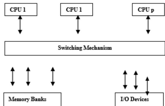
Figure 2: The Uniform Memory Access (UMA) multiprocessor model
