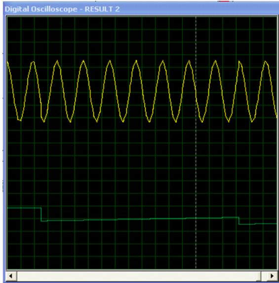
Figure 8: Signal generator implemented by using parallel processing Sine wave Frequency = 1.14 MHz
