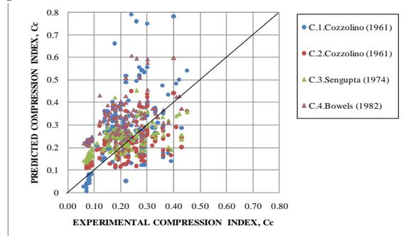
Fig. 3. Comparison of Experimental and Predicted Compression Index ( $C_c$ ) values.
