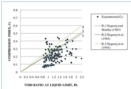
Fig. 2. Compression Index ( $C_c$ ) versus Void Ratio at Liquid Limit ( $e_L$ ).
