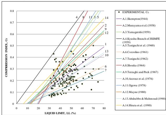
Fig. 1. Compression Index ( $C_c$ ) versus Liquid Limit (LL).
