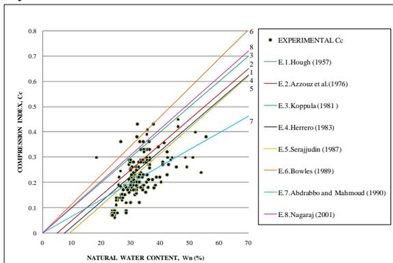
Fig. 5. Compression Index ( $C_c$ ) versus Natural Water Content ( $w_n$ ).
