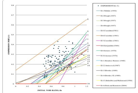
Fig. 4. Compression Index ( $C_c$ ) versus Initial Void Ratio ( $e_0$ ).
