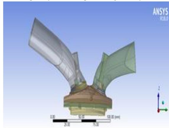
Figure 3.2 Engine Geometry for Cold Flow Analysis
