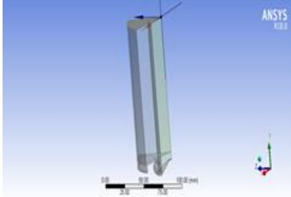
Figure 3.3 Engine Section Geometry for Combustion Analysis
