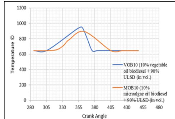
Figure 4.3 Temperature Distribution inside the cylinder at different crank angle for both the fuel
