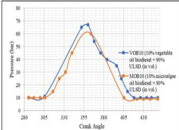
Figure 4.4 Pressure Distribution inside the cylinder at different crank angle for both the fuel
