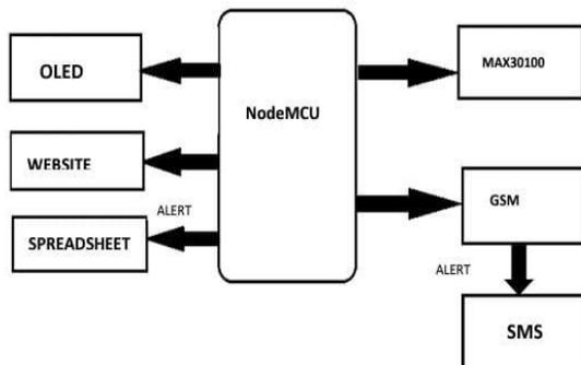
Fig.5.1 BLOCK DIAGRAM
