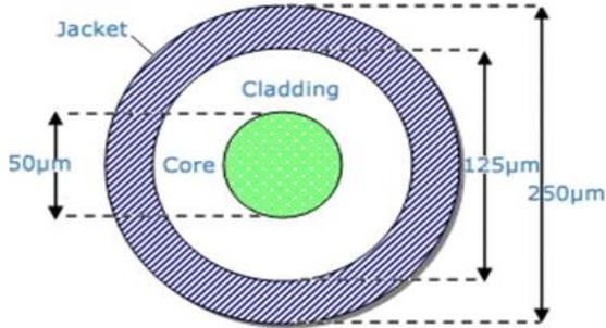
Fig No -1. Cross-section of fibres
