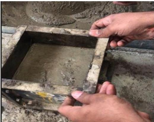
Fig No.5. Placing of Mortar in mould
