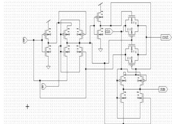
Hybrid Full-Adder (Transistor level)
