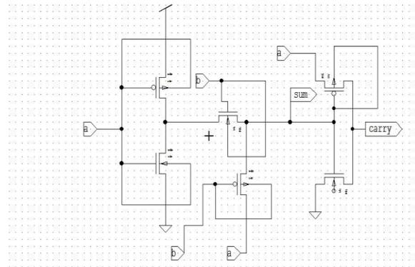
The Proposed design of 6T Half Adder using SG-FinFET
