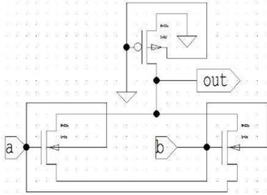
The Proposed design of 3T-AND gate using SG-FinFET.
