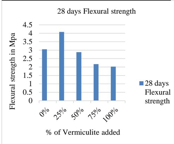
Fig 6.5 Variation of flexural strength for 28 days
