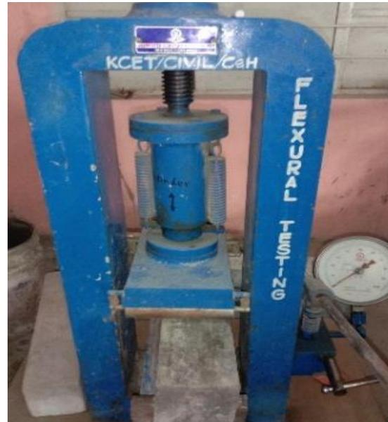
Fig 6.4 Experimental setup for flexural strength test
