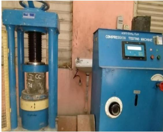
Fig.6.1 Experimental setup for compressive strength of cube
