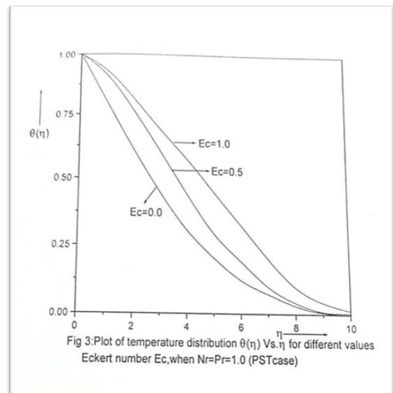
Fig 3:Plot of temperature distribution  $\theta(\eta)$  Vs.  $\eta$  for different values Eckert number  $Ec$ , when  $Nr=Pr=1.0$  (PST case)
