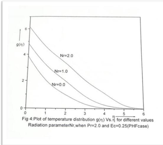
Fig 4:Plot of temperature distribution  $g(\eta)$  Vs.  $\eta$  for different values Radiation parameter  $Nr$ , when  $Pr=2.0$  and  $Ec=0.25$ (PHF case)
