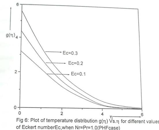
Fig 6: Plot of temperature distribution  $g(\eta)$  Vs.  $\eta$  for different values of Eckert number  $Ec$ , when  $Nr=Pr=1.0$ (PHF case)
