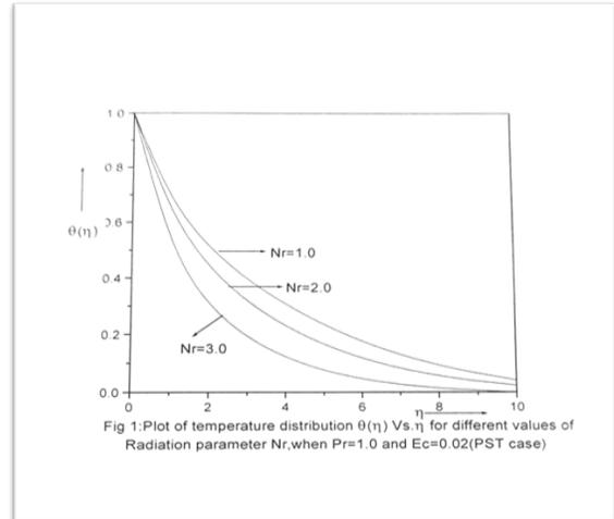
Fig 1:Plot of temperature distribution  $\theta(\eta)$  Vs.  $\eta$  for different values of Radiation parameter  $Nr$ , when  $Pr=1.0$  and  $Ec=0.02$ (PST case)
