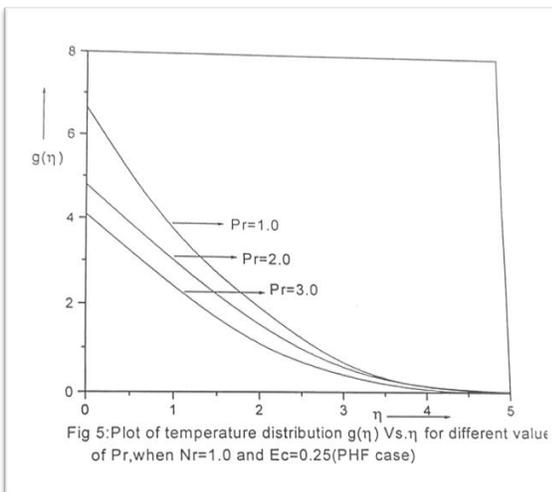
Fig 5:Plot of temperature distribution  $g(\eta)$  Vs.  $\eta$  for different value of  $Pr$ , when  $Nr=1.0$  and  $Ec=0.25$ (PHF case)
