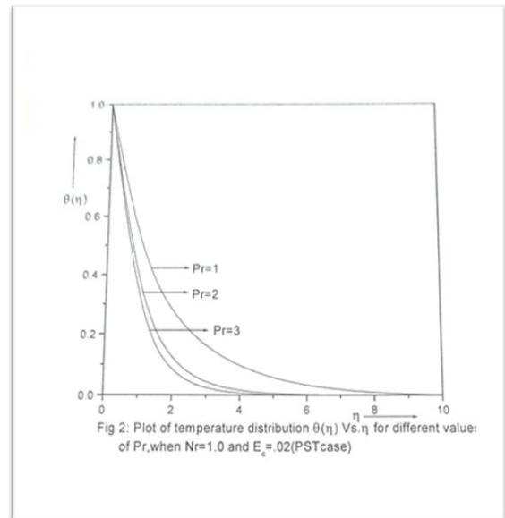
Fig 2: Plot of temperature distribution  $\theta(\eta)$  Vs.  $\eta$  for different values of  $Pr$ , when  $Nr=1.0$  and  $E_c = .02$ (PST case)
