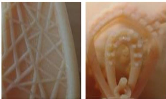
(a) Cleaning and poor surface quality of RPT due to micron range kept on higher side .
