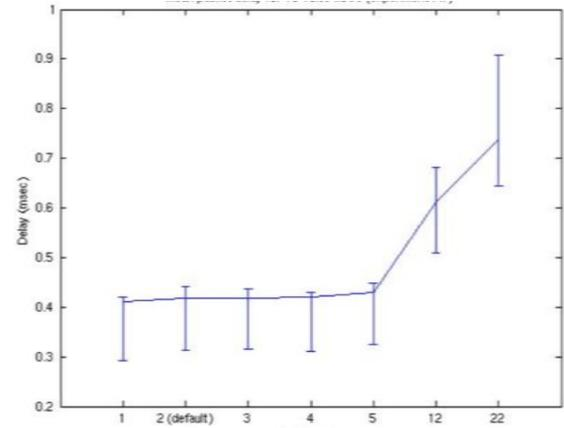
Figure 3: Minimum packet delay for voice flow network, a set of packets synchronously transmitted by the other end point.
