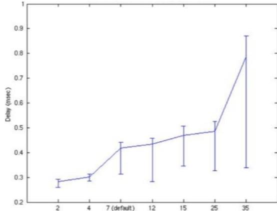
Figure 2: Mean packet delay for voice flows
