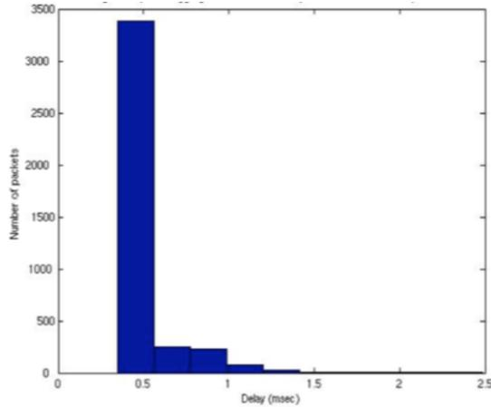
Figure 1: Number of packets delivered at various delay values
